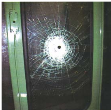
Figure 2: Impact of projectile, penetration of compound design (glass /polycarbon.); source: IWF
